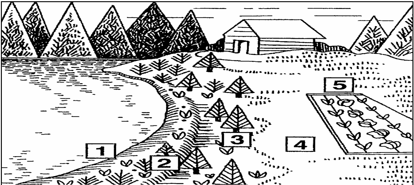
Figure 1. A well designed landscape plan includes 1) and 2) natural vegetation along the water's edge; 3) a natural vegetation filter strip; 4) well-established grass or ground cover; 5) a level flower or vegetable garden set back from the water
